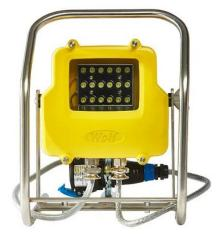
The LinkEx<sup>™</sup> WF-250XL LED Floodlite<sup>™</sup> provides optimal lighting for smaller hazardous area confined spaces using its innovative and patented light engine. It is ideal for 24V applications with limited power supply, allowing up to 8 ATEX LED floodlights to be used in different strings from a single Wolf transformer.
