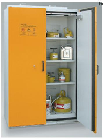
SiS Type 90/1200 VS4 is ideal for storage of flammable liquids at the workplace as per EN 14470-1 (type 90) and TRbF 20 – L. It has automatic thermal closing mechanism if fire occurs. Its outer body is made from powder-coated sheet steel.
