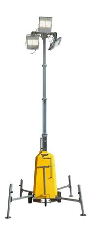
The WTL ATEX Towerlite<sup>™</sup> is a robust, transportable tower light solution certified for ATEX, IECEx, and UKEX Zone 1, 2/21, 22. It extends up to 5.4 meters and features three adjustable LED LFX2 Floodlites, providing up to 78,000 lumens of bright light for illuminating medium to large indoor or outdoor areas.
