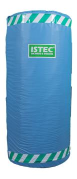
The Protective Cover Against Harsh Weather Conditions is a durable solution designed to protect water tanks from extreme temperature and cold conditions. Its inner aluminum foil fabric and outer polyurethane-coated fabric prevent heat loss and provide effective protection against environmental factors.
